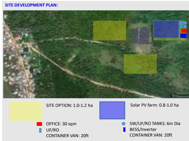
Figure 11. Schematic layout of the development site for the SWRO desalination and PV plant Source: own elaboration
